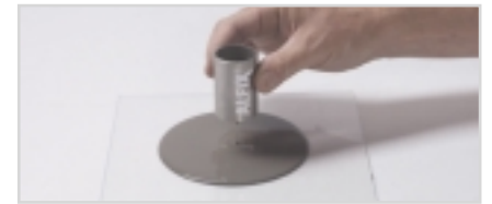
Measuring flow ability
